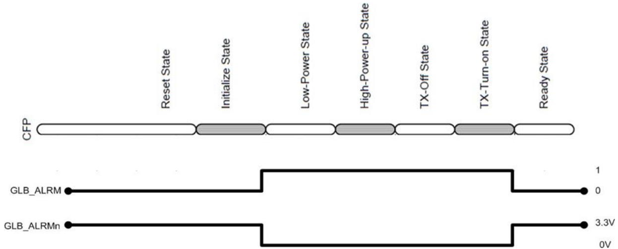
Figure 1: Flowchart for GLB_ALARM Signal
